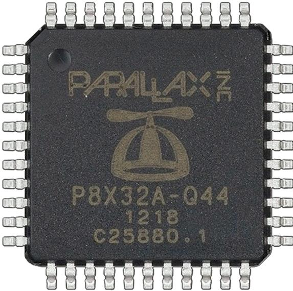
Figure 2.1: The Parallax Propeller microcontroller.
