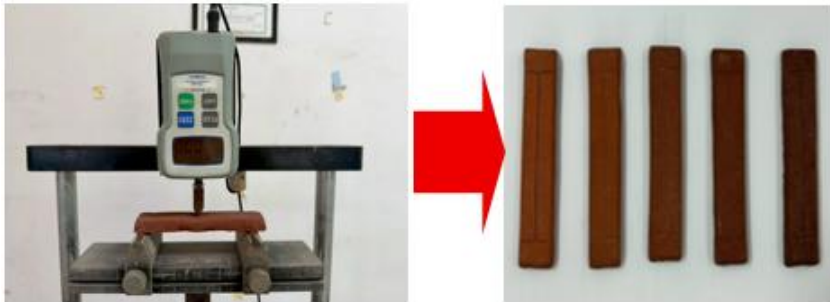
Figure 3. Five Formulations for Ban Kruat Clay Mixed with Pumice Dust Test Strip
