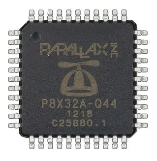
Figure 2.1: The Parallax Propeller microcontroller.
